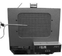
**OUTLET AIR -- Evaporator (Front) Side\***
